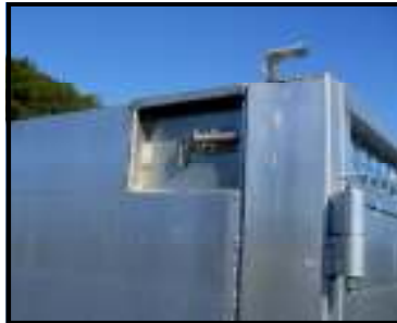
Recessed side wall latches stainless
